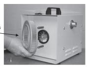
Replace the filter elements and re-assemble in reverse order.
