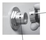
To connect the air hose to the turbine, screw the hose connector onto the outlet of the turbine making sure the thread is not crossed.
