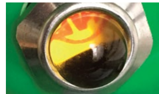
Clearview oil level check
